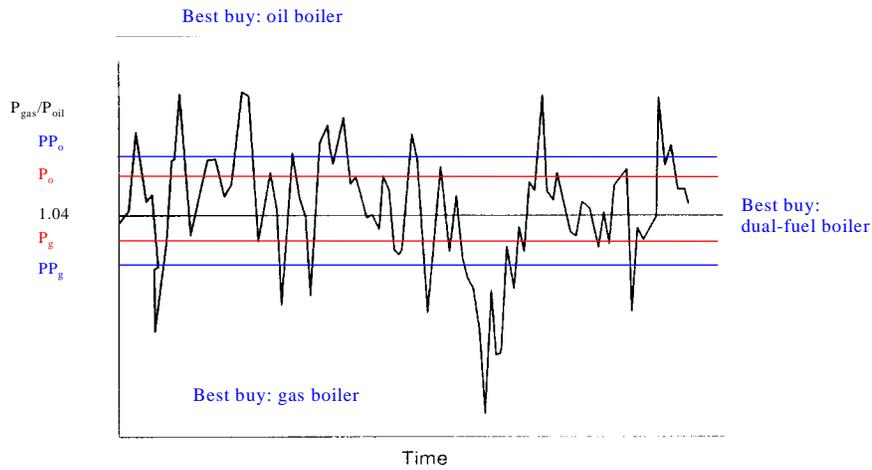
$P_o$  is the fuel price ratio at which the dual burner should be switched to oil when the relative price of gas is going up;  $P_g$  is the ratio at which the dual burner should be switched to gas when the relative price of gas is going down. The gap between  $P_o$  and  $P_g$  increases with the cost of switching and with volatility.
